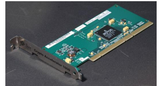
Encryption: PCI-X Crypto Accelerator
