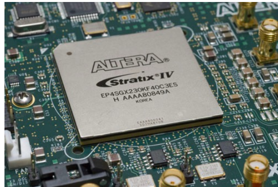
Generic FPGA: A Stratix IV FPGA from Altera
