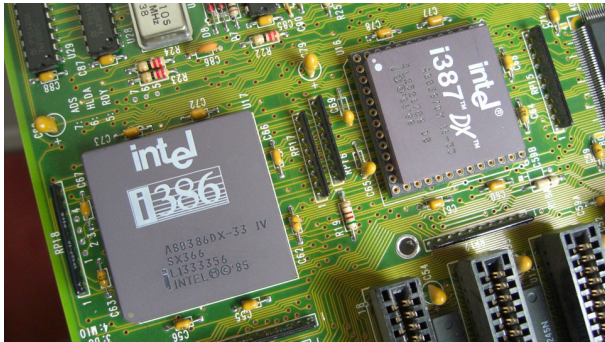
Computation: Intel 80386DX CPU with 80387DX Math Coprocessor
